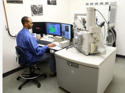
Focus Ion Beam/Scanning Electron Microscope
