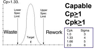
Use the problem solving process to identify and prevent the root causes of waste (usually below the lower specification limit) and rework (usually above the upper specification limit). The goal, is to reduce variation so that all of your points fit within the specification limits, clustered around a target.
